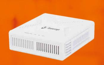
S-XPON-1001-ONT (1GE+CATV ONU) is support Dual mode (EPON and GPON), It can also be applied to a wide temperature environment, and also has a powerful firewall function.
